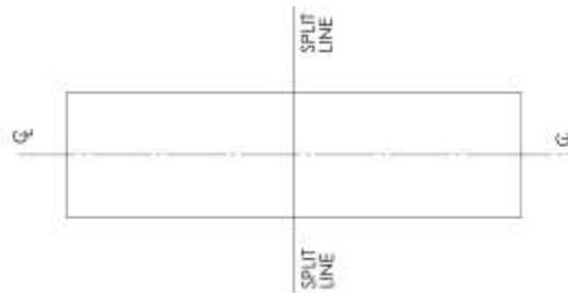
Check that there is sufficient room below the panel for the housings and the location is either flat or with minimal radius. Place the template onto the panel. Line up the split lines on the template with the panel edge. Mark around the cut-out and remove the template.
